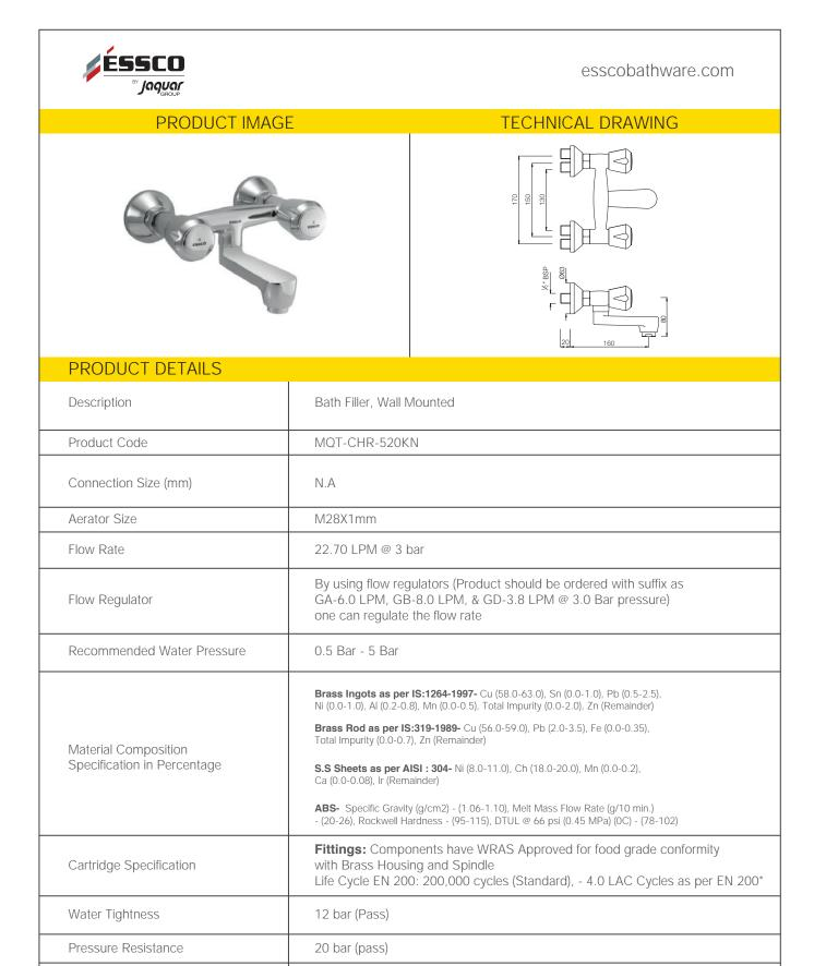
**Plating:** Nickel-8.0 micron Chromium-0.20 micron, Salt Spray 300 hrs + Validated), Adhesion (Pass)
